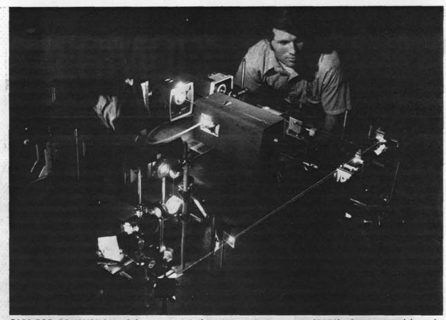
CARS FOR COMBUSTION-Coherent Anti-Stokes Raman Spectroscopy (CARS), demonstrated here by Larry Rahn of Applied Physics Division 8342, is one of the methods of laser diagnostics being developed for combustion studies at SLL. The technique gives high resolution, strong signals, and good rejection of fluorescent light, advantages which make CARS useful in measuring temperatures and species concentrations in combustion environments.
